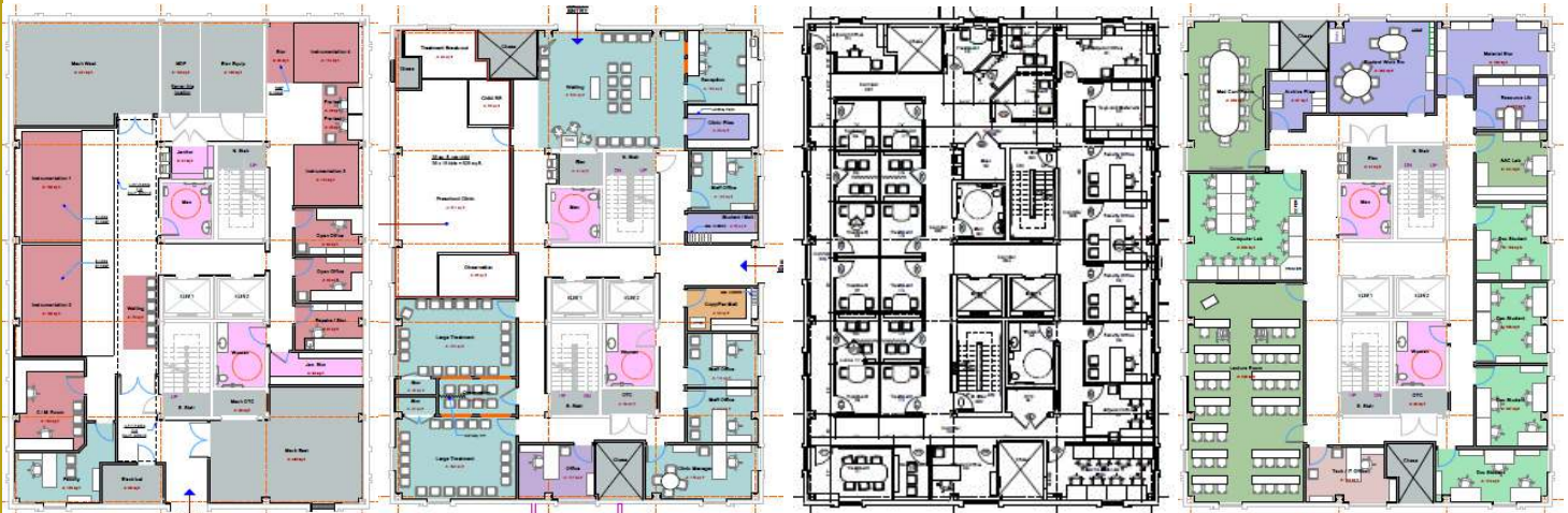
(L-R) Basement (audiology testing), 1st Floor (Clinic/Observation), 2nd Floor (Offices, Doc Rooms) 3rd Floor (Student Spaces)
